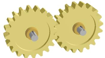
A simple gear train uses two gears, which may be of different sizes. If one of these gears is attached to a motor or a crank then it is called the driver gear. The gear that is turned by the driver gear is called the driven gear.
