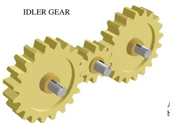
When a simple gear train has three meshed gears, the intermediate gear between the driver gear and the driven gear is called an idler gear.
