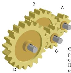
Compound gear trains involve several pairs of meshing gears. They are used where large speed changes are required or to get different outputs moving at different speeds.
