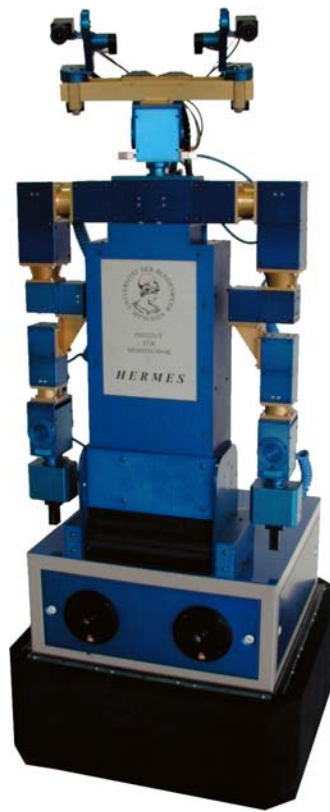
Figure 2: Humanoid experimental robot HERMES ; mass: 250 kg; size: 1.85 m · 0.7 m · 0.7 m
