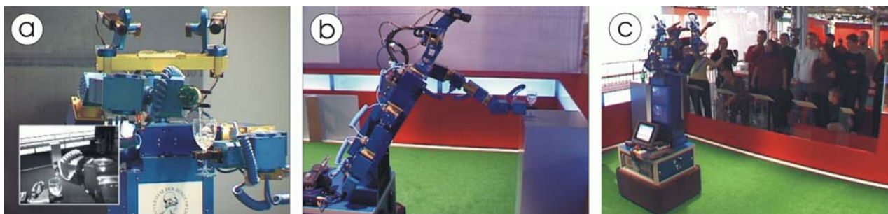
Figure 11: HERMES performing at the special exhibition "Computer.Brain", instructed by commands given in natural language: taking over a bottle and a glass from a person (not shown), filling the glass with water from the bottle (a); driving to, and placing the filled glass onto, a table (b); interacting with visitors (here: waving with both arms, visitors wave back!) (c)
