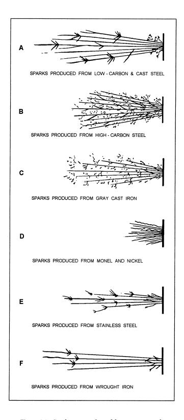
Figure 1-4.—Spark patterns formed by common metals.
