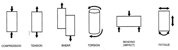
Figure 1-1.—Stress applied to a material.
