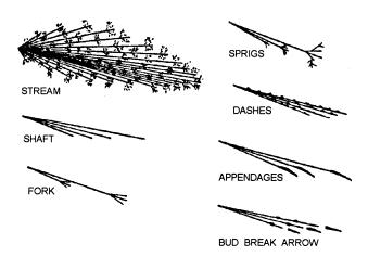
Figure 1-2.—Terms used in spark testing.
