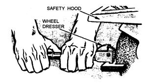
Figure 1-3.—Using a grinding wheel dresser.
