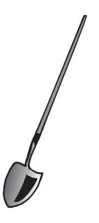
long or short with a straight shaft or a D-shaped handgrip. The choice of handle style depends on personal preference; long handles offer greater leverage and are less tiring to use in many cases.
